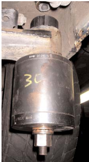
Photo #2 Extracting old bushing
