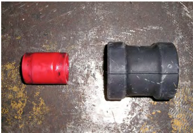
ST urethane mount vs. M5 hard rubber mount
