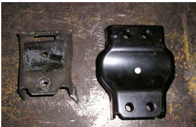
ST urethane mount vs. M5 hard rubber mount
