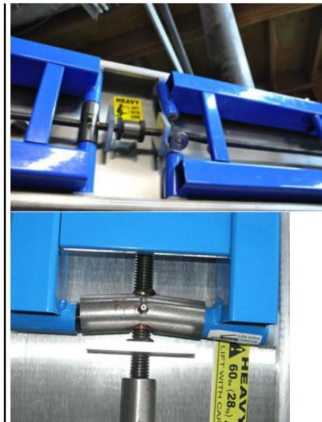
They will break if extremely overloaded. This will prevent from hurting the operator and damaging major components of the lift. Once the safety snaps, the lift will drop between 1 and 1.5 inches and will scare the heck out of you. It can and should not hurt anyone unless you have your hands and feet right under the lift when it shifts down.
